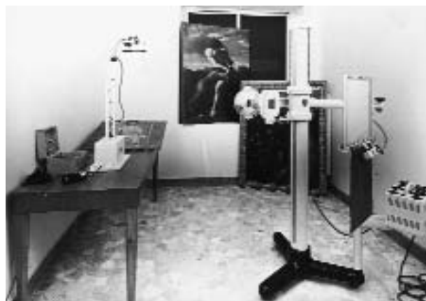
FIG. 3. An examination room with equipment for X-radiography and an ultraviolet lamp at Studio d'Arte Palma.
